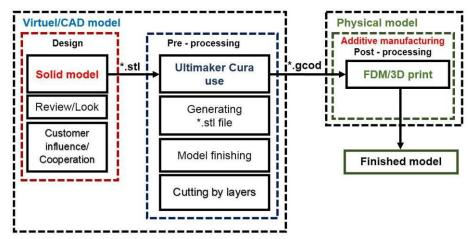
Figure 1: Block diagram of model/prototype realization
