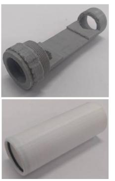
Figure 6: Electronics enclosure elements made on a 3D printer
