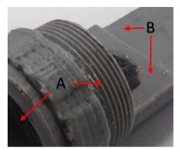
Figure 7: Additional machining on the lathe: thread (A) and contact surface (B)
